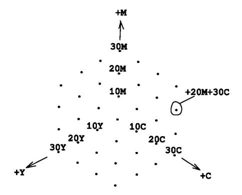
A joint color and brightness test is a net spread over the logical region around an initial guess, to catch the right exposure.
