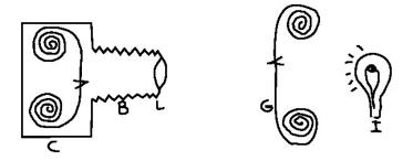
It consists essentially of a camera (C) connected by a bellows (B) to a lens (L) aimed at a film in a gate (G) illuminated from behind by a lamp (I).
