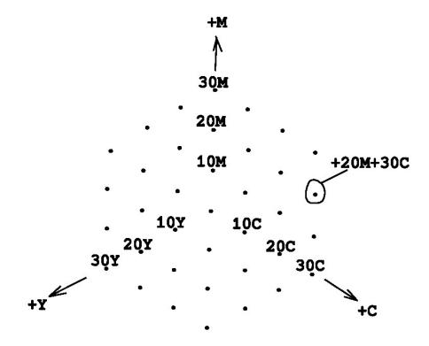
A joint color and brightness test is a net spread over the logical region around an initial guesea, to catch the right exposure.
