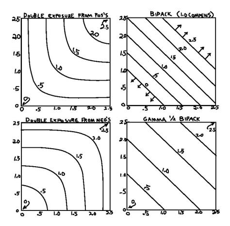
For a double exposure it doesn't matter which exposure is first, or what time separates the two. In some multi-head optical printers, using a beam-splitter, the two exposures are simultaneous. Either way, the two films can be independently adjusted for exposure, filtered, etc.
