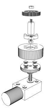
The choice to direct drive the take-up is due to the fact that powerful geared DC motors are cheap and available. Driving them separately, rather than using a belt, means that the speed can be controlled individually but that they do not need to. The speed of one take-up can be set to expect a daylight spool but could be adjusted in future work to optimize for a 2 or 3 inch core.
