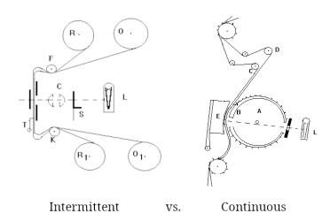
Contact printers can be continuous or intermittent-motion: meaning that they expose each frame individually, pausing for each exposure. This project will create a continuous printer for simplicity. Intermittent-motion printers require precise movements, more complex lamps or shutter mechanisms and would make this a more complicated DIY project. This is to be avoided for now.
