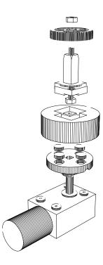
The choice to direct drive the take-up is due to the fact that powerful geared DC motors are cheap and available. Driving them separately, rather than using a belt, means that the speed can be controlled individually but that they do not need to. The speed of one take-up can be set to expect a daylight spool but could be adjusted in future work to optimize for a 2 or 3 inch core.
