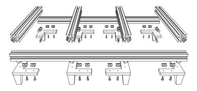
It would be possible to increase the rigidity, if needed, by adding additional intermediary crossing lengths but for this prototype a total of six (6) lengths connected by five (5) panels and eight (8) corner brackets has been sturdy enough for all tests.
